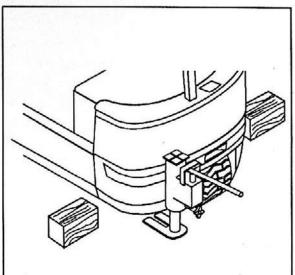
Once the truck is jacked up, place a wood block under each side of the rear counterweight and lower the truck onto the blocks.
