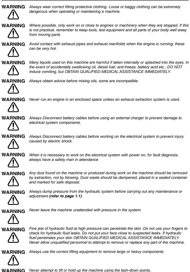
Never attempt to lift or hold up the machine using the lash-down points.
