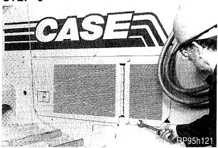
Remove the right and left hand side screens for the engine compartment.
