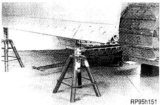
Raise and block the dozer blade up. Use a floor jack to support the undercarriage guards and remove the guards from under the engine and torque converter.
