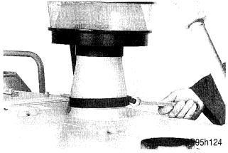
Loosen the clamp holding the inlet stack and precleaner for the air intake and remove the inlet stack.
