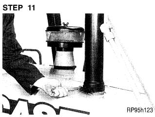
Loosen the clamp holding the exhaust pipe and remove the exhaust pipe.
