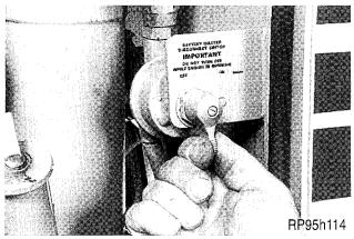
Turn the master disconnect switch for the battery to the OFF position.
