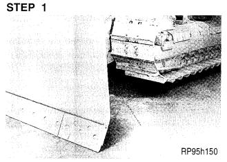
Place the crawler on blocks at least 8 inches high to allow the C-Frame to drop below the bolts mounting the radiator shroud. Alternate Method is to remove the dozer blade and C-Frame as an assembly.
