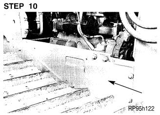
Remove the right and left hand lower side shields for the engine compartment.
