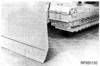
Remove the blocking from under the dozer blade and lower dozer blade to the floor.
