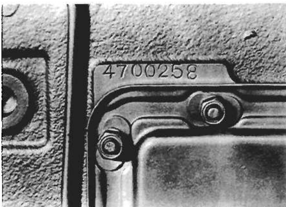
Engine Number Location (4.236 Phase I Type)
