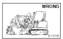
Always lower the bucket and blade to the ground before doing any maintenănce.
