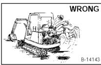
Keep body, jewelry and clothing away from moving parts. away from moving parts, electrical contact, hot parts and exhaust.
