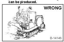
Stop, cool and clean engine of flammable materials before checking fluids.
