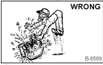
Lead-acid batteries produce flammable and explosive gases. Keep arcs, sparks, flames and lighted tobacco away from batteries.
