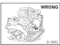
A Stop, cool and clean engine of flammable materials before checking fluids.
