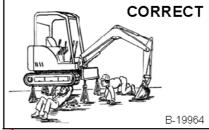
Luse the correct procedure to lift and support the excavator.
