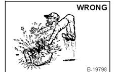
Lead-acid batteries produce flammable and explosive gases.
