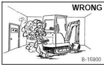
Vent exhaust to outside when engine must be run for service.
