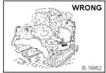
Stop, cool and clean engine of flammable materials before checking fluids. Never service or adjust machine
