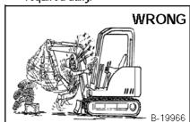
Always lower the bucket and blade to the ground before doing any maintenănce. Never modify equipment or add attachments not approved by Bobcat Company.
