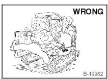
Stop, cool and clean engine of flammable materials before checking fluids. Never service or adjust machine
