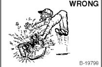
Lead-acid batteries produce flammable and explosive gases. Keep arcs, sparks, flames and lighted tobacco away from batteries.
