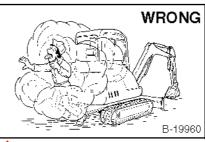
Vent exhaust to outside when enaine must be run for service. Exhaust system must be tightly sealed. Exhaust fumes can kill
