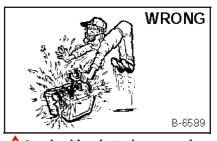
Lead-acid batteries produce flammable and explosive gases. Keep arcs, sparks, flames and lighted tobacco away from away batteries.
