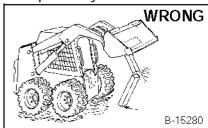
Never work on loader with lift arms up unless lift arms are held by an approved lift arm support
