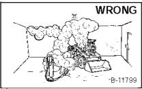
ventilation when good welding` grinding parts. Wear dust mask when grinding
