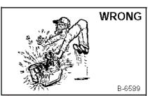
produce Lead-acid batteries flammable and explosive gases. Keep arcs, sparks, flames and lighted tobacco away from
