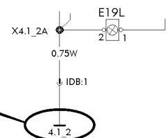
Earth connection point 4, earth connection 1 and wire 2.
