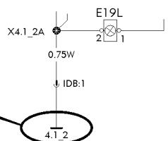
Earth connection point 4, earth connection 1 and wire 2.
