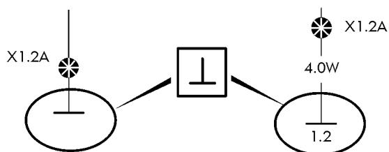
Same splice can be drawn on several diagrams. The wire from the splice to the earth connection point will only be drawn and coded on one diagram. On the other diagrams will only the earth connection point be written besides the splice.
