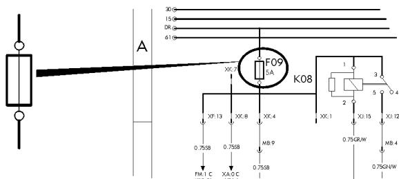
Reference arrow, for diagram BA, coordinates 0 C, component A17, connector PA pin 29.
