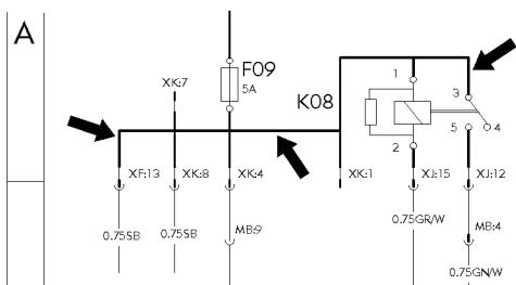
Conductor on circuit card.
