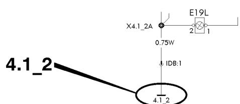
Earth connection point 4, earth connection 1 and wire 2.
