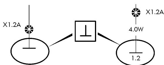
Same splice can be drawn on several diagrams. The wire from the splice to the earth connection point will only be drawn and coded on one diagram. On the other diagrams will only the earth connection point be written besides the splice.
