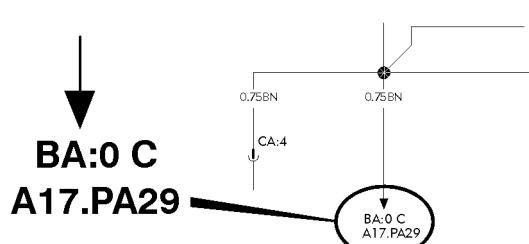
Reference arrow, for diagram BA, coordinates 0 C, component A17, connector PA pin 29.
