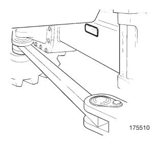
The Syncro Shuttle serial number is stamped on a label which is mounted to the rear face of the unit.
