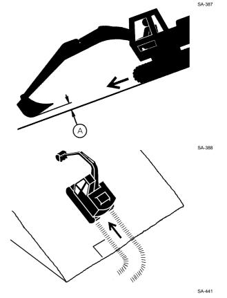
Driving across the face of a slope or steering on a slope may cause the machine to skid or turnover. If the direction must be changed, move the machine to level ground, then, change the direction to ensure sage operation.
